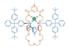
Chloride wins: A new, versatile chloride-anion-templating synthetic pathway is exploited in the preparation of a series of eight new [2]rotaxane host molecules (see image), including the first sulfonamide interlocked system. <sup>1</sup>H NMR spectroscopic titration investigations demonstrate the rotaxanes' capability to recognise chloride anions in competitive aqueous solvent media, including a dicationic rotaxane that binds chloride in 35% water.
