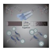
Nanotube detergents: Deep insights into the arrangement of various surfactants noncovalently bound to the sidewall of single-walled carbon nanotubes (SWCNTs, see figure) have been obtained by analysis of the sedimentation coefficients with analytical ultracentrifugation. The investigation included classical detergents, as well as synthesized perylene-based surfactants.
