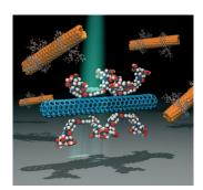
Nanotube surfactant design: The interactions of synthesized perylene-based surfactants with single-walled carbon nanotubes (SWCNTs) of various diameters have been investigated. The surfactants exhibit an enhanced adsorption affinity towards smaller-diameter SWCNTs (see figure), which could be of great importance for future nanotube separation by selective dispersion.
