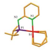
Selective amine alkylation: The synthesis of eight new iridium complexes containing anionic P,N ligands (see image) is described. These new complexes were used as highly active catalysts for the selective monoalkylation of anilines with primary alcohols, and gave nearly quantitative conversion under mild reaction conditions.
