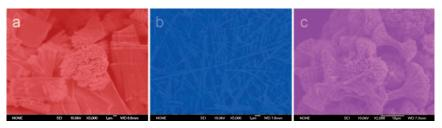
How do your crystals grow? Morphology control of  $Sb_2S_3$  crystals (see figure) could be realized by using a solution-phase route, through manipulating the interaction between the sol-
